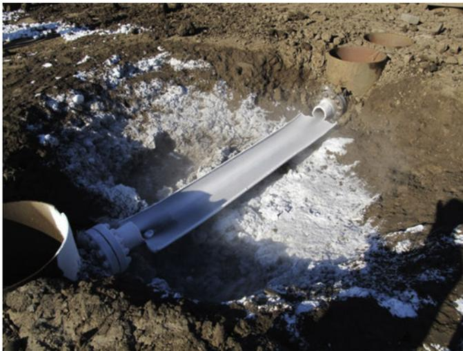
Fig. 16. Photograph of the crater and ruptured pipe.
